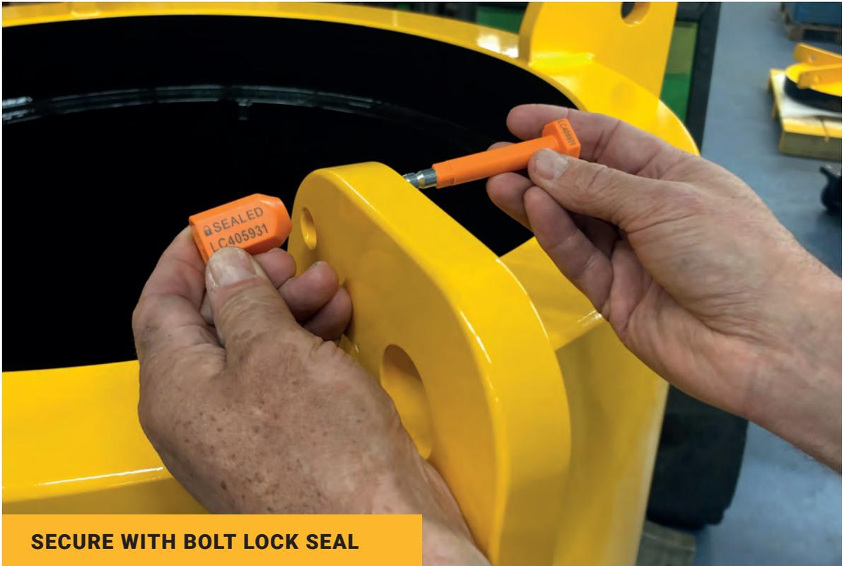
**SECURE WITH BOLT LOCK SEAL**
